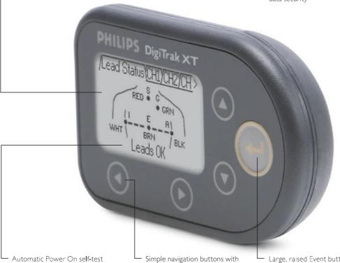
Automatic Power On self-test with onscreen status indicator guarantees reliable recording Simple navigation buttons with tactile response for fast setup
