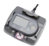
Fast downloads typically take less than 90 seconds. Our dual dock accepts DigiTrak XT and DigiTrak Plus recorders.
